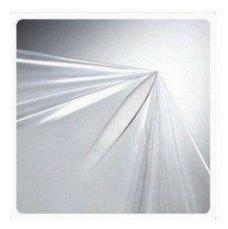
After the invention of Metallocene PE, the gap for high quality shrink film narrowed. MPE has very good dart drop strength, elongation, holding force and considerable shrink ability. This resulted in use of thinner films compared to LDPE. For example 120 micron film of LDPE can easily be replaced by 80 micron MPE film. This resulted in considerable saving in packing cost with added strength and protection in packing. MPE shrinks fast in low temperature and does not become saggy after cooling.
